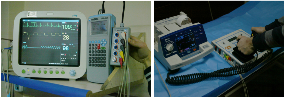
Fig. 11. The performance measurements of the patient monitor and the defibrillator
