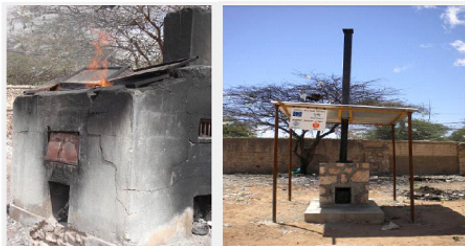
Pic. 13. 'De Montfort' incinerators
