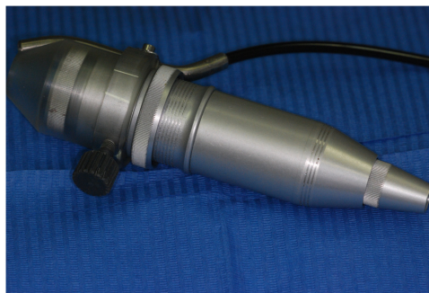
Fig. 20. Specially designed Nd: YAG laser tip for intraoral metal welding. (Courtesy of Prof. Carlo Forniani)
