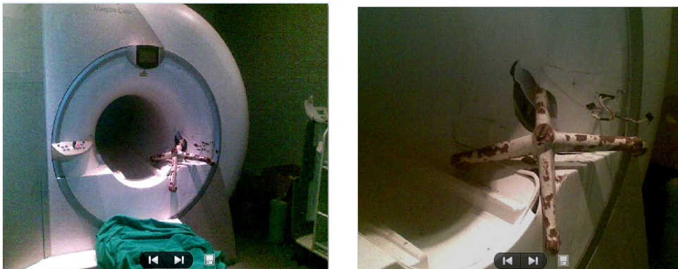
Fig. 5. Photographs of a hanger of saline physiology stuck to the MRI (Sezdi, 2009a)
